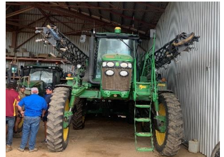
Figure 10 - Wide wheeled machinery, straddles 2 cane rows and suits multiple peanut rows. Narrow tyres reduce damage to the peanut crop
