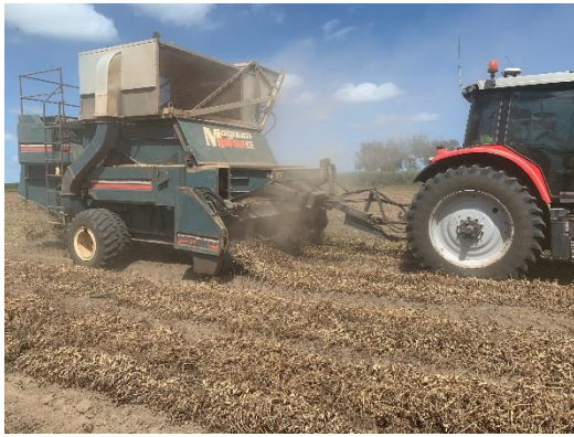
Figure 7 - A tow behind thrasher and all in one machine
