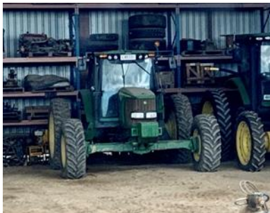
Figure 10 - Wide wheeled machinery, straddles 2 cane rows and suits multiple peanut rows. Narrow tyres reduce damage to the peanut crop
