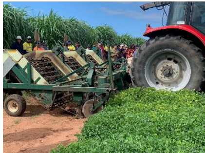
Figure 5 - Left to right, 2 row digger, KMC 6 row digger and fluffer
