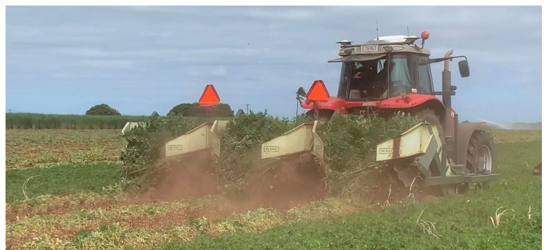
Figure 6 - KMC 6 row digger in action
