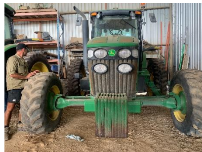
Figure 10 - Wide wheeled machinery, straddles 2 cane rows and suits multiple peanut rows. Narrow tyres reduce damage to the peanut crop
