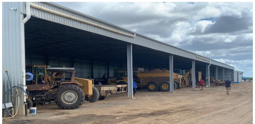
Figure 10 - Wide wheeled machinery, straddles 2 cane rows and suits multiple peanut rows. Narrow tyres reduce damage to the peanut crop
