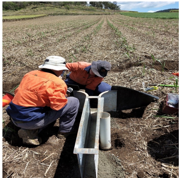
Image: SRA staff Molly O'Dea and Matt Schembri installing one of the six flumes at the Balnagowan demonstration site.
