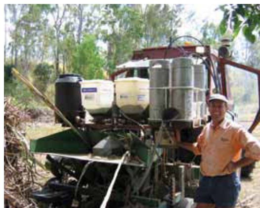
Image 9 | Equipment used by BSES for planting insecticide trials with a double-disc opener planter; two granular products could be applied from the Microband boxes which were driven by an electric motor connected to either one with a removable collar, while four liquid treatments could be applied from the pressurised canisters.
