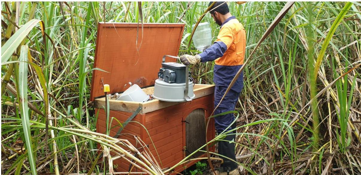
Figure 2: Automatic samplers collected water samples into a 9 L jar from which sub-samples were collected and sent for analyses.
